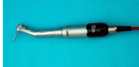
**The handpiece is connected to the coupling of the micromotor. When reaching the final position both parts will be lock. To unlock, the conta- angle handpiece is pulled off from the micromotor.**
