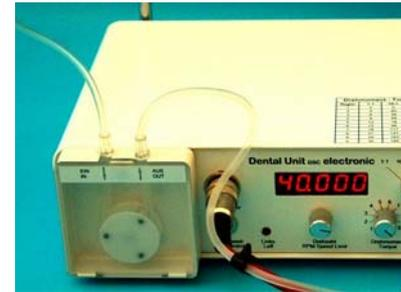
**Please pay attention to the IN- and OUT direction when inserting the hose fitting for the coolant fluid. Optimumfunktion of the coolant pump is guaranteed only, if the original hose fitting of HKM is used.**
