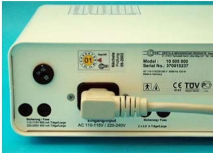
Prior to the connection of the power cable, it has to be checked, that the voltage switch(15) is set to the country´ s specific voltage. If this is not the case the voltage switch has to be adjusted with a screwdriver or a small coin to the country´ s specific voltage.
