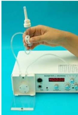
After opening the coolant pump housing(12) the non-sterile assistant places the reinforced part of the hose fitting with slight tension around the pump rotor and fixes it into the the slotted holding device. Then the spike of the drip chamber is inserted into the bottle with coolant fluid.
